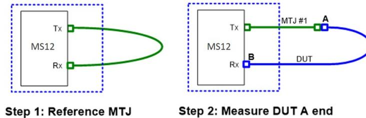
Figure 3- Typical testing sequence with MS12001
